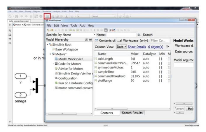
The outputs of the motor command conversion subsystem which are the left and right wheel velocities are fed to the '**ZumoMotors**' block. The '**ZumoMotors**' block represents the motors on the assembled Zumo Robot.
