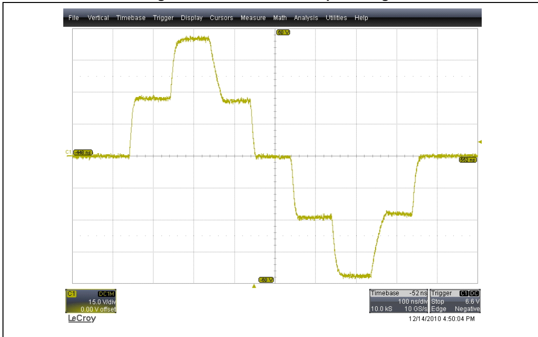
Figure 14. Five-levels HV output voltage
