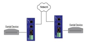
Figure 14. Paired Mode Setup
