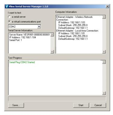
Figure 18. Testing a VCOM Port
