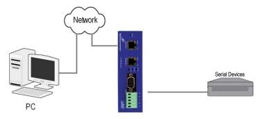
Figure 13. Direct IP and Virtual COM Port Connection
