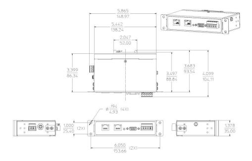
Figure 20. Dimensional Diagram of a VESR321 Serial Server
