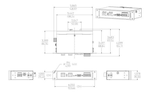
Figure 21. Dimensional Diagram of a VESR321 Serial Server
