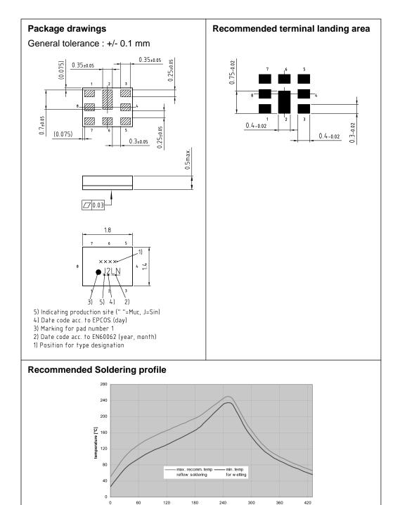
for Convection and Infrared Soldering - Lead-free
