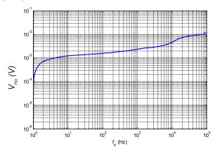
Figure 3: Output noise, cumulated rms
