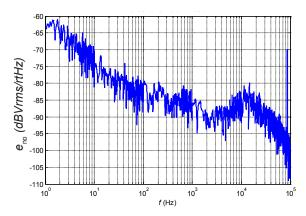
Figure 2: Output noise voltage spectral density
