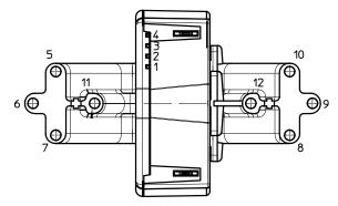
The four integrated primary conductors have a diameter of 2.5 mm. The three conductors 5-10, 6-9 and 7-8 could be used as the lines in a three phase system; the conductor 11-12 could be used either as the neutral in a three phase system or as a test current conductor.
