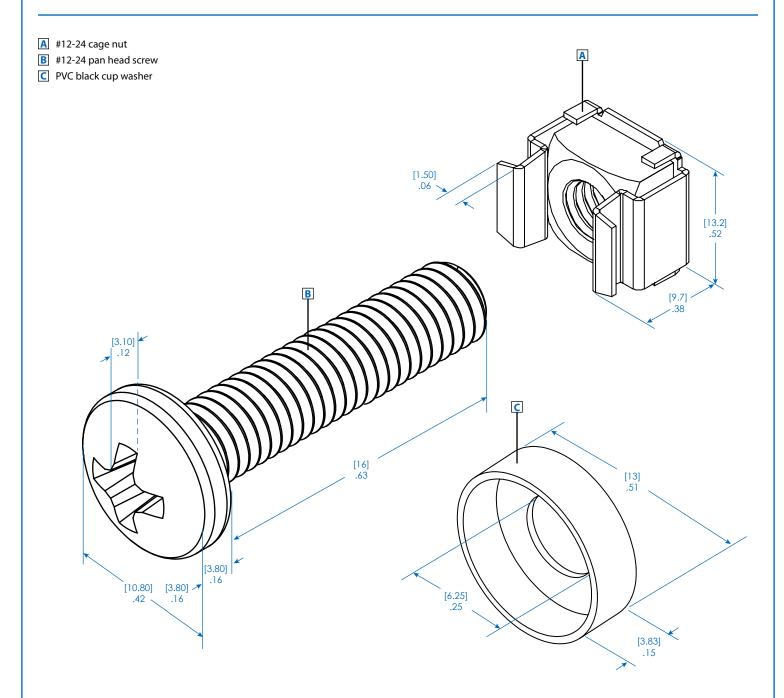
• Square hole hardware kit contains 50 each #12-24 pan head screws, #12-24 cage nuts and PVC cup washers
