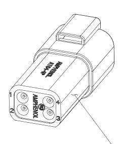
RECEPTACLE, 4 PIN, AT SERIES, REDUCED DIA. WIRE SEAL
