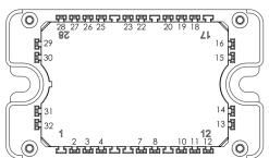
Pins 29/30/31/32 must be shorted together Pins 26/27/28/22/23/25 must be shorted together to achieve a phase leg
