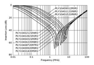
Differential Mode Insertion Loss-Frequency Characteristics
