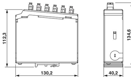
DIN rail splice box 6x LC duplex OM4, fully mounted ready to splice
