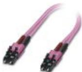
Assembled FO cable, zip cord cable, multi-mode fiberglass 50/125  $\mu\text{m}$ , OM4, plug: LC/LC, degree of protection: IP20, for installation in cable ducts or control cabinets
