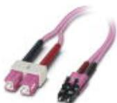
Assembled FO cable, zip cord cable, multi-mode fiberglass 50/125  $\mu\text{m}$ , OM4, plug: SC/LC, degree of protection: IP20, for installation in cable ducts or control cabinets
