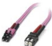
Assembled FO cable, zip cord cable, multi-mode fiberglass 50/125  $\mu\text{m}$ , OM4, plug: LC/SC-RJ, degree of protection: IP20, for installation in cable ducts or control cabinets
