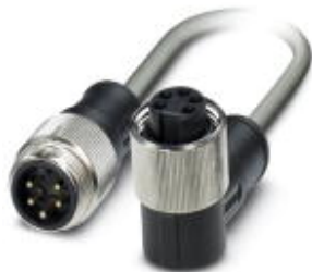
Bus system cable, DeviceNet, 5-position, PUR halogen-free, Gray RAL 7001, Plug straight 7/8"-16UNF, on Socket angled 7/8"-16UNF, Cable length: 1 m
